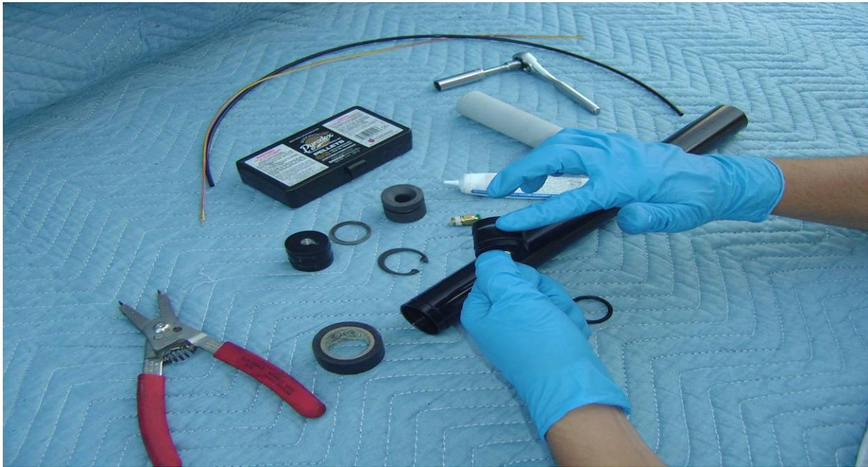
**Step 3:** Use Krytox™ grease on top Bulkhead O-rings. Smear Krytox™ over the entire outer cylindrical surface of the Bulkhead. This allows for an easy fit into the motor case. Krytox grease is available from Conrail Rockets and our Dealers.
