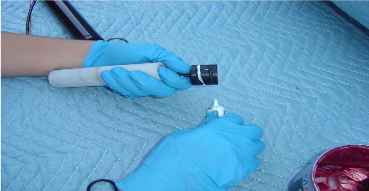
**Step 10:** Now that the Injector and Igniter assembly is put together, you will be greasing the Injector Assemble with Krytox™ Grease just as you did with the top bulkhead. Once the Injector is greased you will slide the assembly into the motor tube. Be sure to not slide the injector up to far, as you will use the grain to push the injector up the rest of the way into the case.
