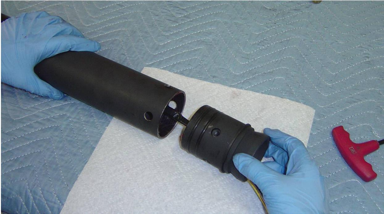
**Step 9:** Grease the Nozzle O-rings and slide the nozzle into the combustion chamber. If you will be using a retaining ring on the nozzle, be sure to put this onto the nozzle prior to bolting it into the combustion chamber.
