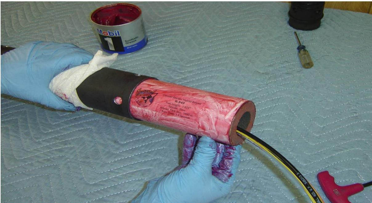
**Step 8:** Grease the included fuel grain with a synthetic type grease (Mobile 1 or similar) and slide the fuel grain into the combustion chamber. Ensure that the fill lines, vent line and igniter wires are all drawn through the core of the grain. A thin coating of grease is all that is required.
