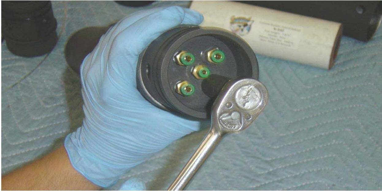
**Step 3:** Insert Press Lock Fittings into the Injector Face. A 1/8 Inch Fitting will always go in the center port. 1/8 inch Fittings are used for Slow Motors, 3/16 for Medium Motors and 1/4 Inch for Fast Motors. The Fittings should be tightened 1/2 turn past tight.
