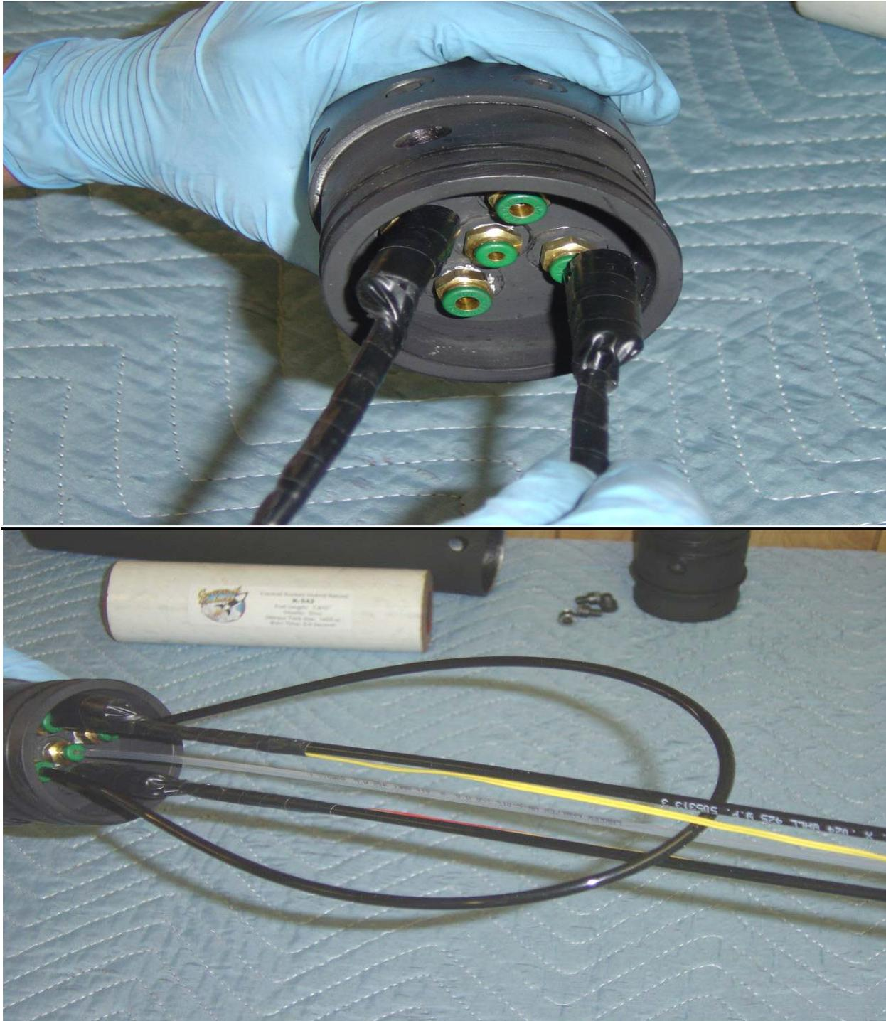
**Step 5:** Insert the Fill lines w/ Pyrodex Pellets attached into the injector baffle on opposite sides. Ensure that the nylon lines go all the way into the press locks and go past the O-Ring Seal. You will feel it go past the O-ring and seat at the bottom of the fitting. You will now insert the clear vent line into the center fitting, and the short crossover line into the last 2 fittings. Ensure that all the lines are secure in the fittings prior to moving on.
