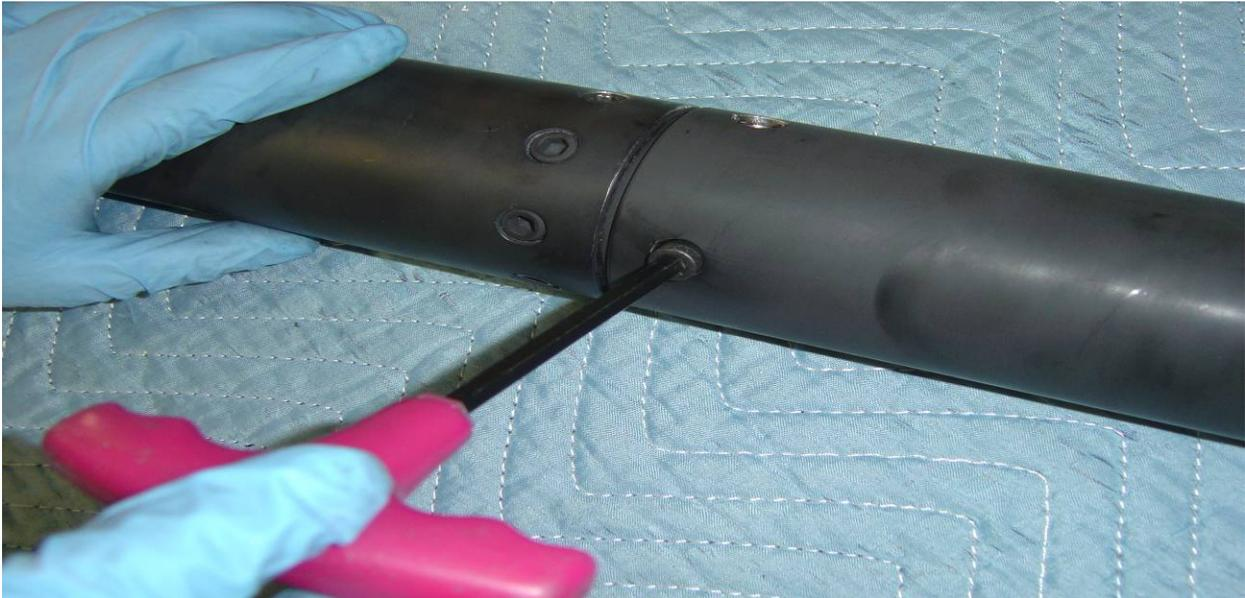
**Step 7:** Grease the Injector Baffle O-rings and slide the nitrous tank section of the motor onto the combustion chamber and insert the retention bolts. The bolts will require a 1/4 inch hex head wrench.
