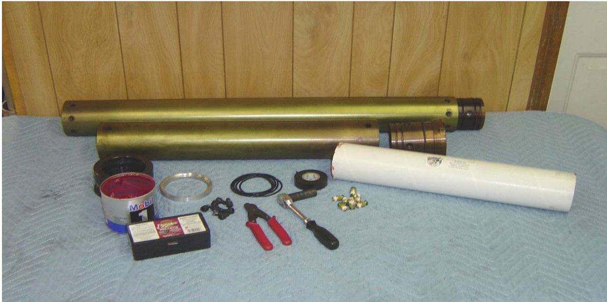
**Step 1:** Ensure that your motor hardware is clean and free from grease, oils, dirt and debris. Wipe the motor components with soap and water, to cut any residual grease from previous firings. Make sure you have all required tools and parts for motor assembly.
