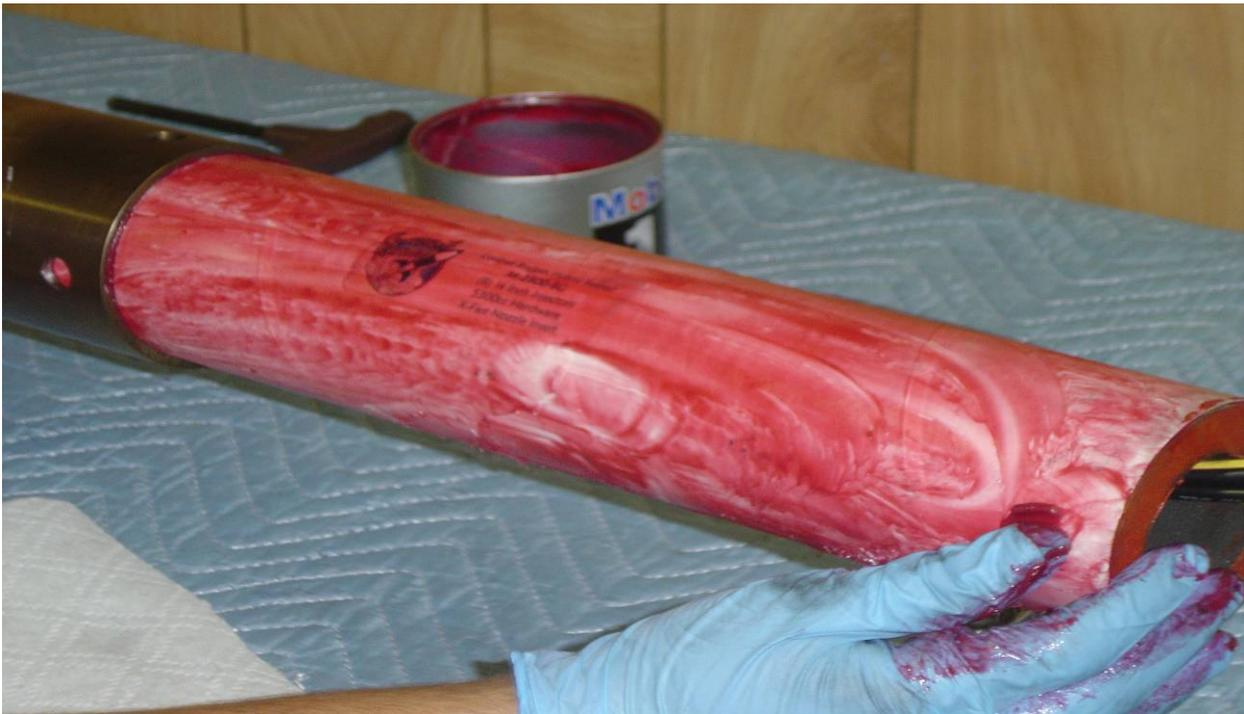
**Step 8:** Grease the included fuel grain with a synthetic type grease (Mobil 1 or similar) and slide the fuel grain into the combustion chamber. Ensure that the fill lines, vent line and igniter wires are all drawn through the core of the grain. A thin coating of grease is all that is required.
