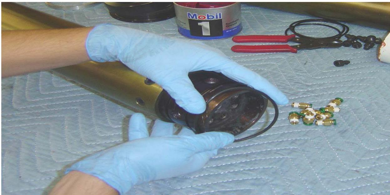
**Step 2:** Begin by installing all O-Rings onto Nozzle and Injector Baffle. All O-rings are Dash Number 236. O-Rings should be free from any cracks, burns or damage.
