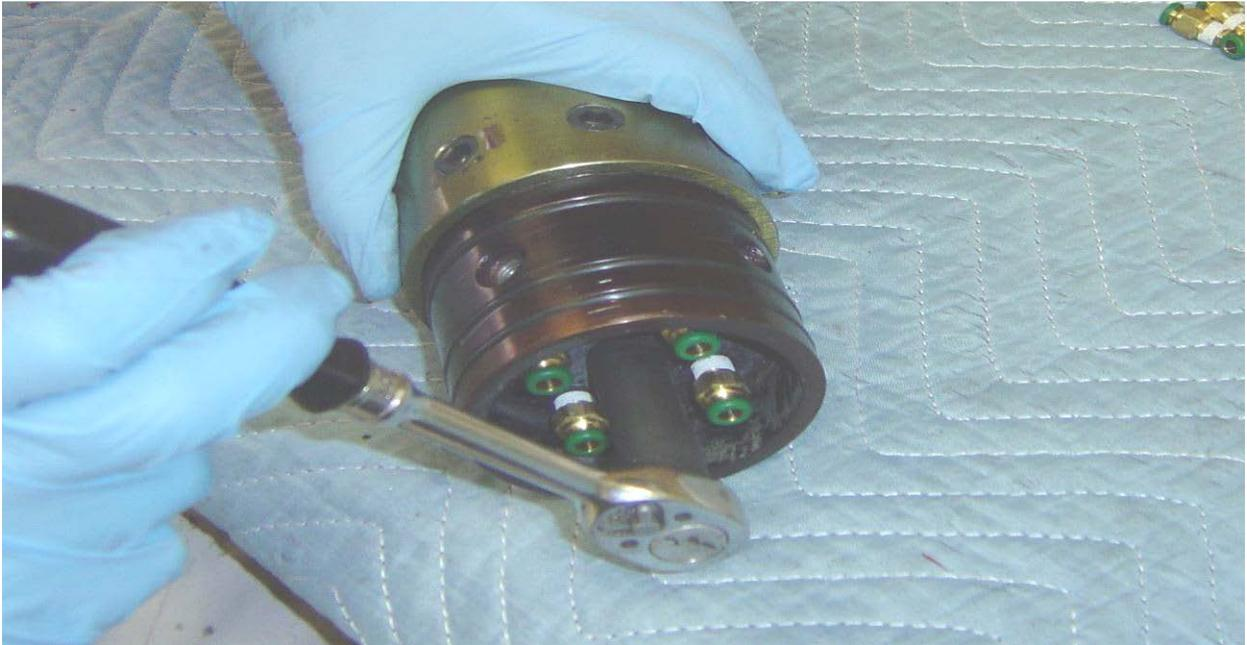
**Step 3:** Insert Press Lock Fittings into the Injector Face. A 1/8 Inch Fitting will always go in the center port. The Fittings should be tightened 1/2 turn past tight. If only 4 Injectors are used (Slow and Medium Motors) the Injectors should alternate radically with a steel plug. (4 Steel Plugs will be included with the necessary reloads)
